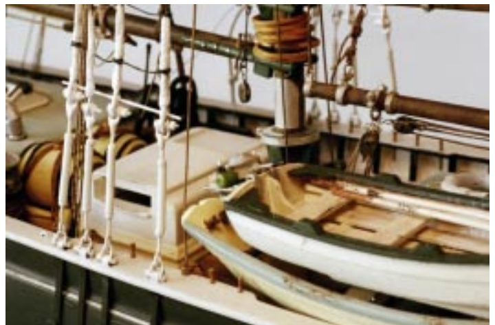
The turnbuckles. Also note the dory and skiff with attached Evinrude outboard motor.
