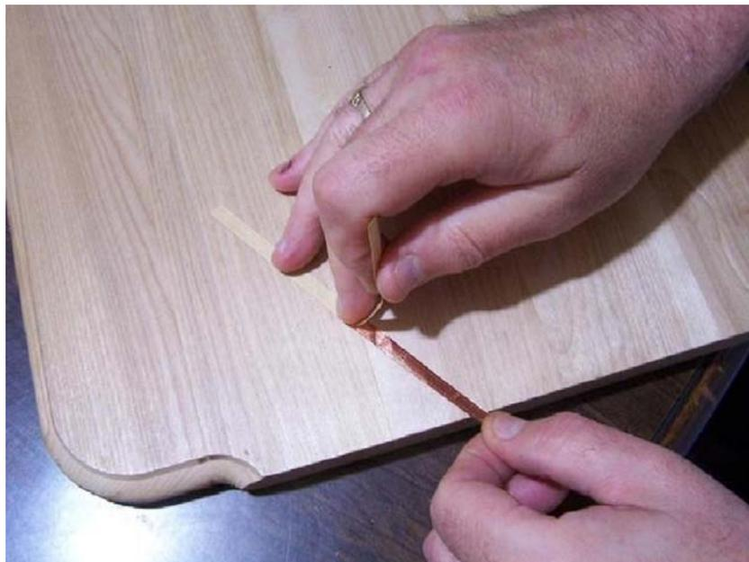
7. The best place to install the first strip of copper is at the stern-most edge of the bottom of the keel. So, using both hands, attach the copper strip there. Make sure it is centered, even, and has no wrinkles. It can still be lifted with an X-Acto knife to make adjustments at this point. Once you are satisfied, press it down
