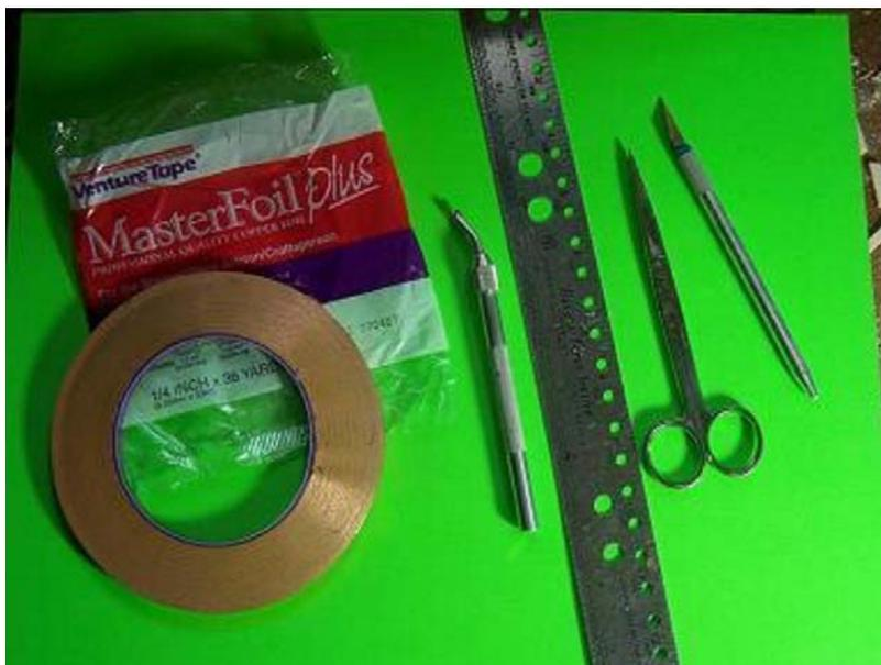
5. **Thin Steel Ruler:** It must be thin enough so that the pounce wheel turns effectively and makes the proper impression in the copper tape.
