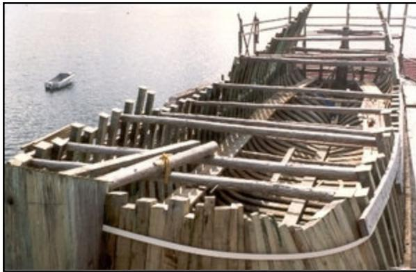
Dubbing of the side frames in order to fair the ship to accept hull planking was completed. Transom pieces were fitted and modified, filling pieces and most inserts were installed and the deck beams were dubbed as with the side frames to accept the deck plank. The installation of hanging knees to the deck beams and ceiling under the main deck commenced as far as material would allow.
