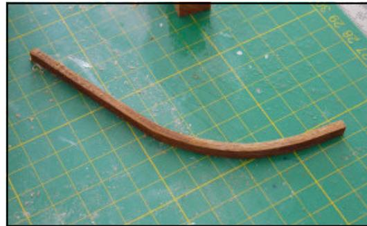
I place the planks in room temperature water for about 10 minutes to soak a bit. Then I start to fondle it with hot iron's ending nob. Immediately you will see and hear the steam going from the wood.
