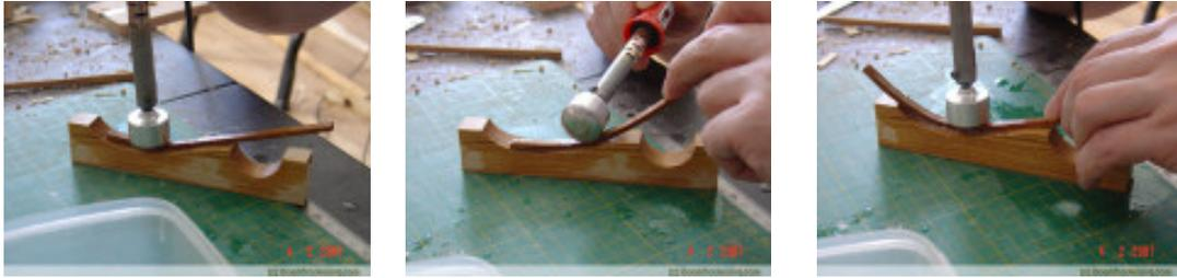
And then of course I keep on pressing and releasing and so on until I am happy with the result. Aha, I forgot about something. The plank will get dry after few minutes so from time to time I soak it with water again only to make it wet on the surface. When the plank is 80% pre-shaped and still a bit wet position it on the hull and clamp it to dry fully out but in correct bent position.
